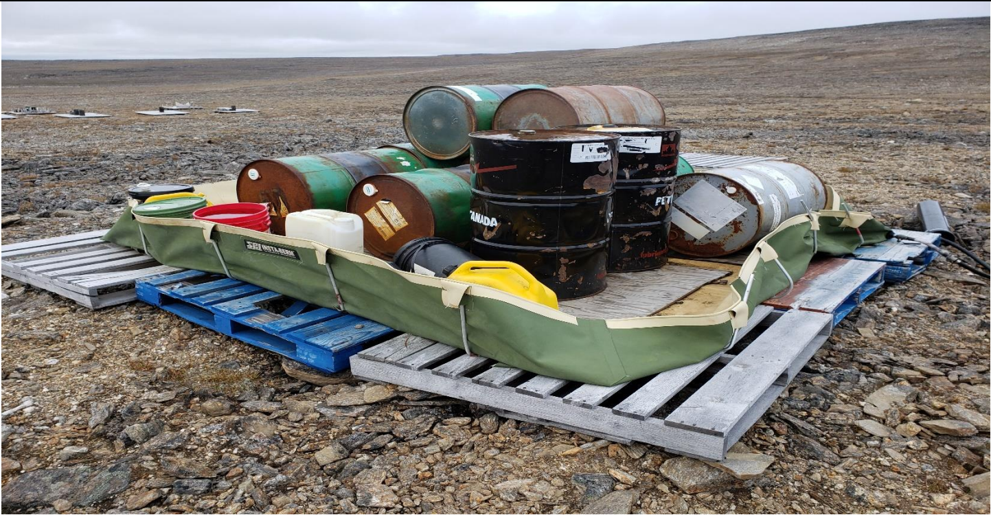
Description: fuel cache in secondary containment. Spill Kit Observed in close proximity. Walls compromised. Secondary containment did not contain any liquid.
