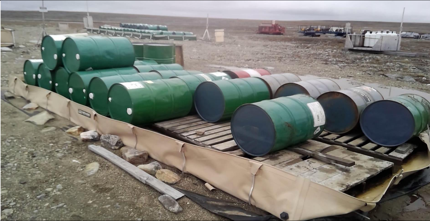
Description: Discovery Camp - Fuel Cache 1 – 26 barrels of Jet-A fuel in secondary containment
