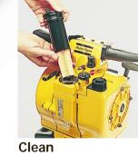
Easy access to the air filter means dust particles can be removed in seconds.
