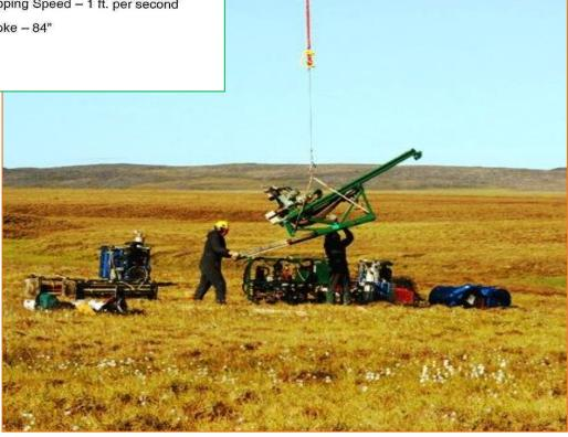
The drill and ancillary equipment totals approximately 12,500 lbs with the heaviest lift being 1250 lbs. A total of 12 loads using a Long Ranger. The drill and equipment fit comfortably in 4 Twin Otter loads. They drill with one 12 hour shift per day and can average 1 hole per day including moves once routine is established.
