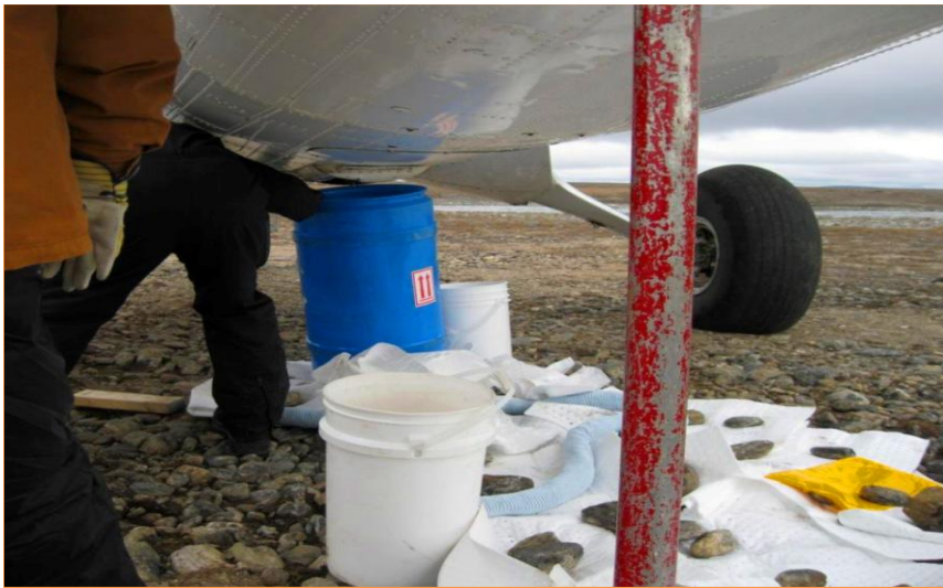
Left: Spill-kit drum, pails captured 25L immediately. Above: Spill pads on fuel trail.
