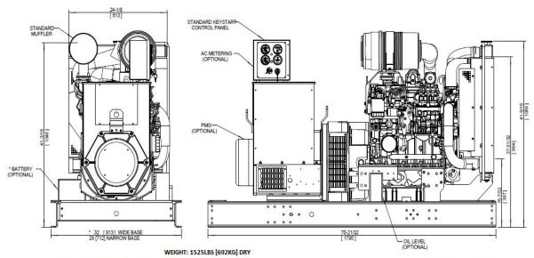
FUEL TANK, ENCLOSURE AND BATTERY TRAY AVAILABLE WITH A 32 [813] WIDE SKID ONLY
