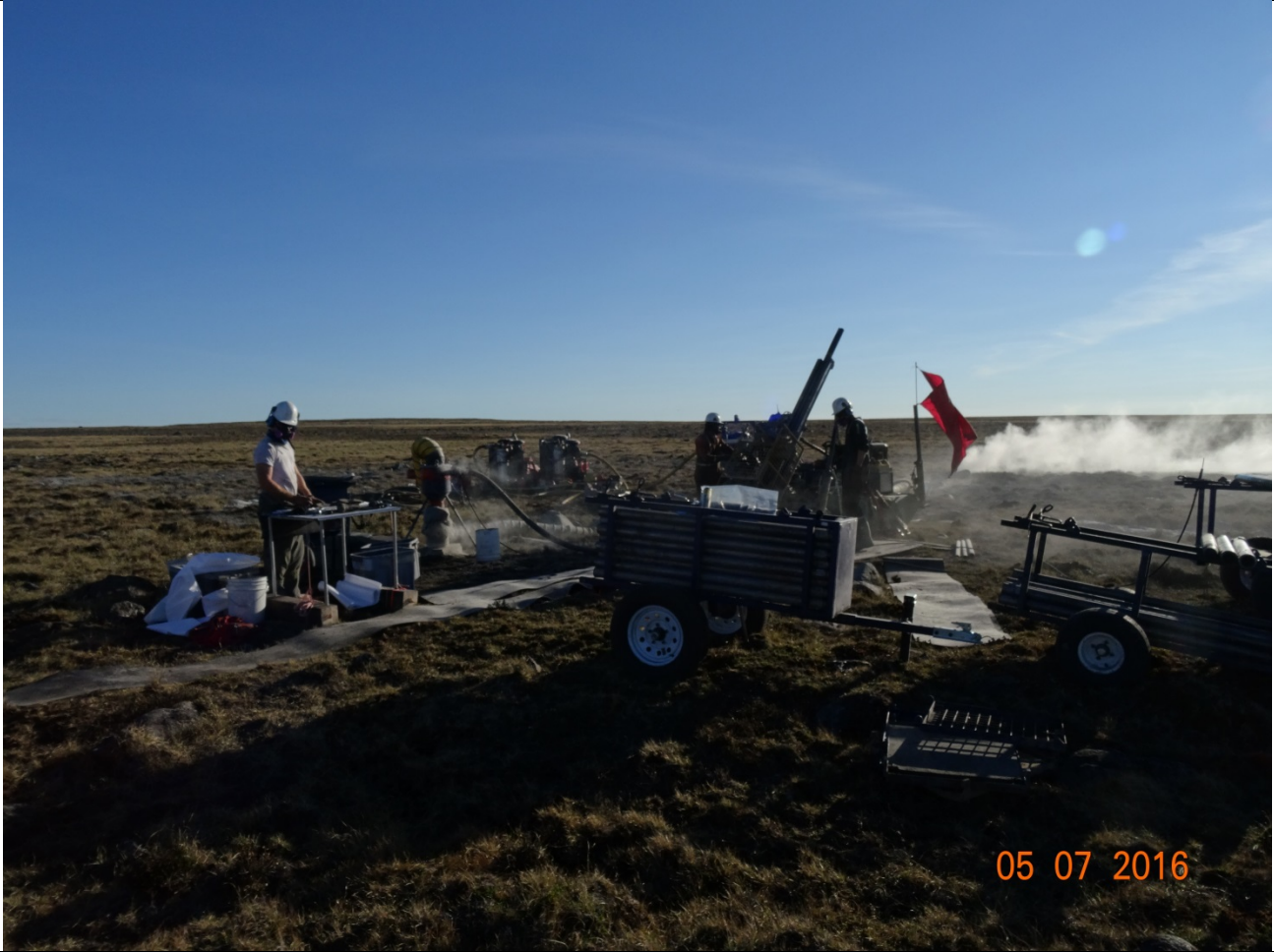
Description: Active RAB setup at hole 35. Chemicals/oils all in containment.
