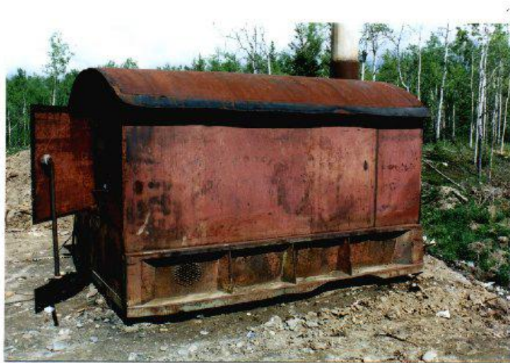
Figure 2 – Enclosed Metal Burn Box Photo courtesy of Alaska Department of Environmental Conservation
