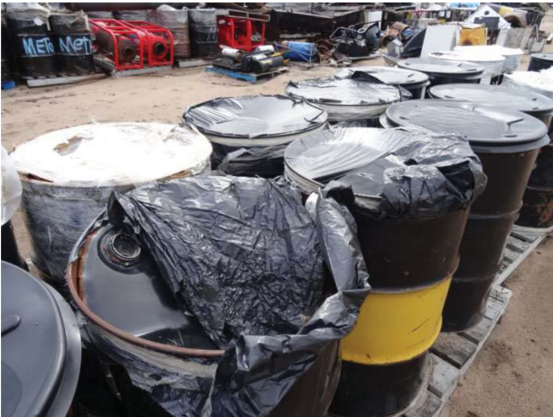
Figure 4. Barrels are no longer sealed.
