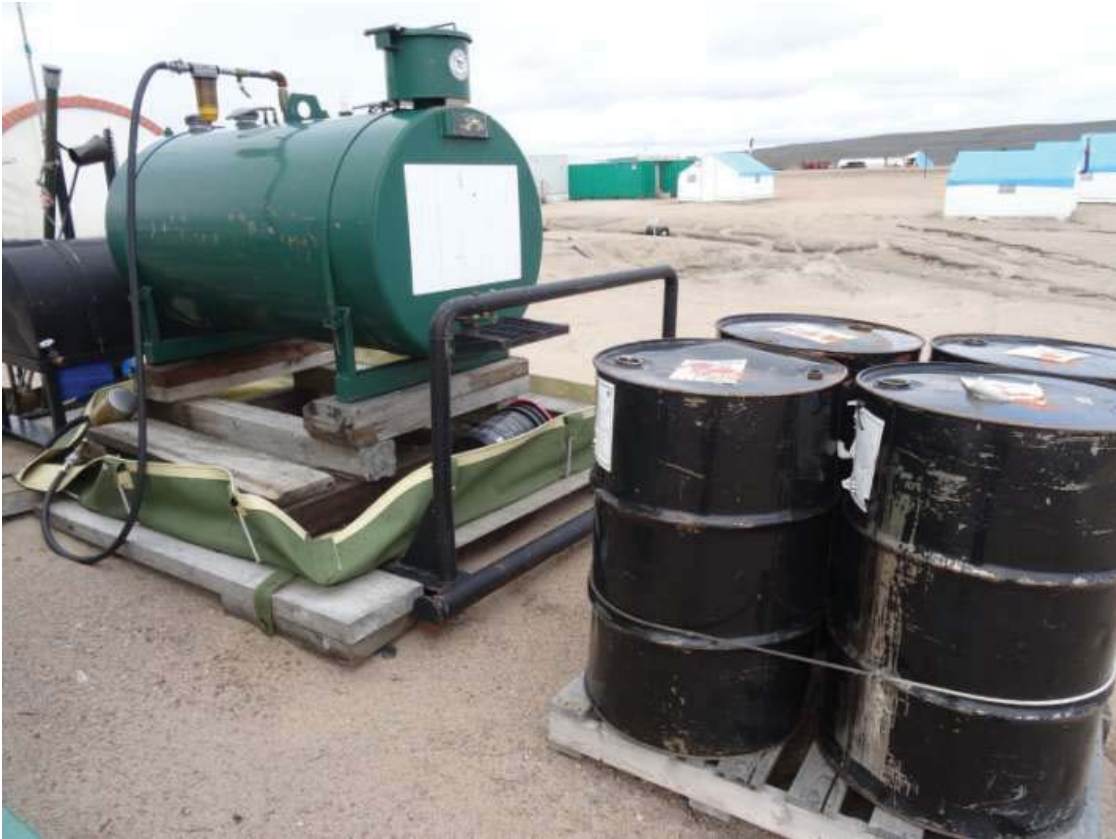
Figure 21. Barrels out of containment at the incinerator.
