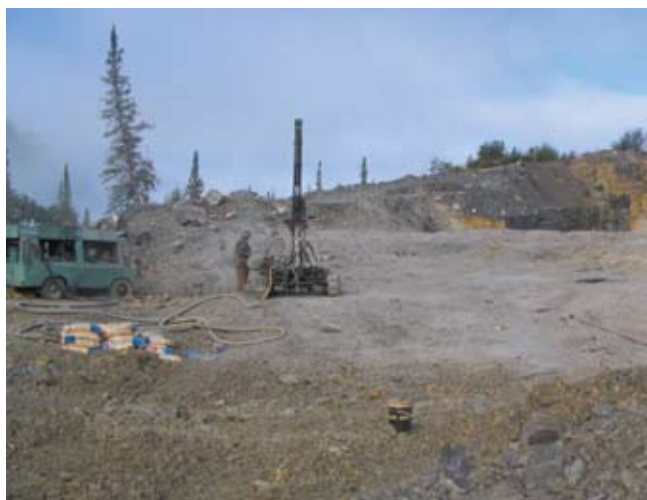
FIGURE 22. Extraction of rock involves drilling and blasting.
