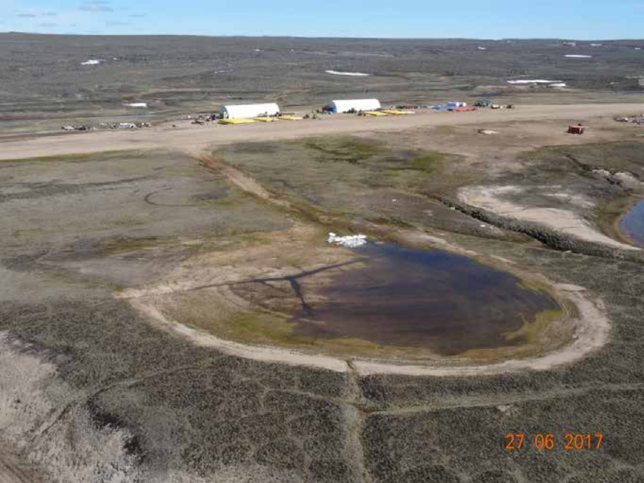
Description: Borrow Area 1 is accumulating water. Historic drainage paths can be seen.
