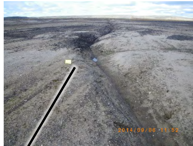
Melted ice wedge shows signs that steady state conditions may have developed
