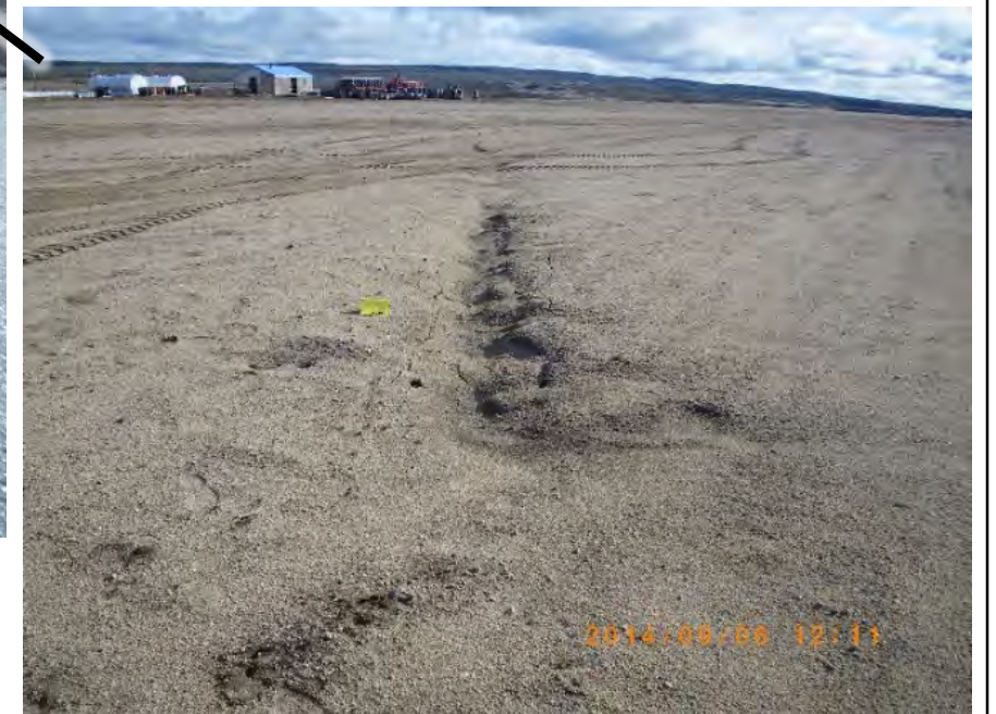
No further melting of the ice wedge suggests steady state conditions have developed
