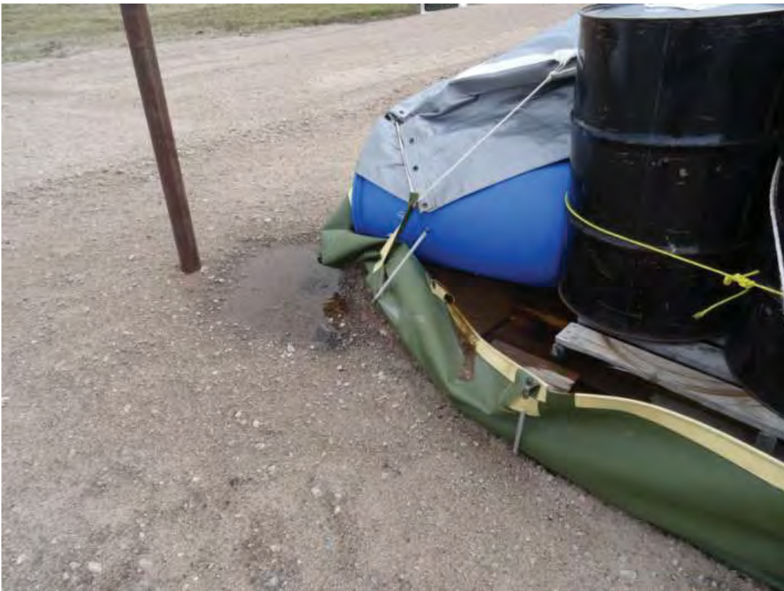
Figure 26. Hayes Camp berm; corner dripping. No obvious contamination at this time.
