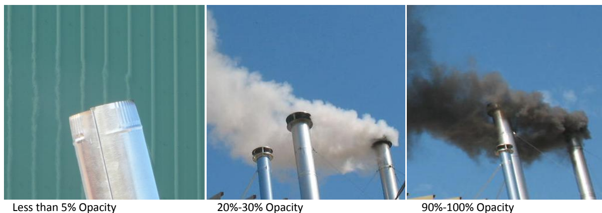
Figure 6 - Examples of Smoke Opacity Ratings
