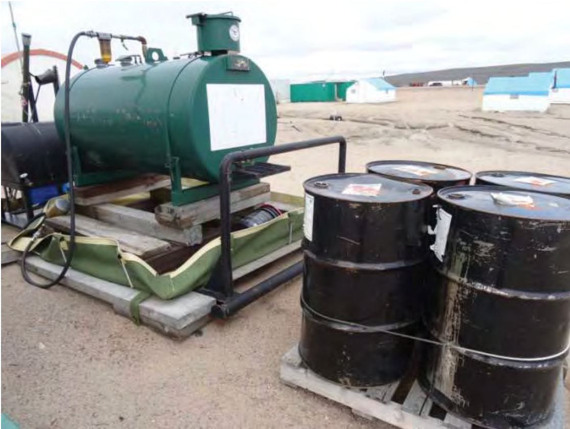
Figure 21. Barrels out of containment at the incinerator.
