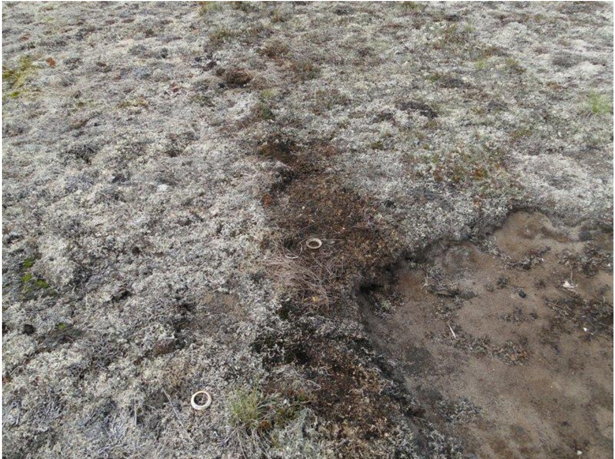
Figure 7. Hydrocarbon staining still visible, and excavation was not backfilled.
