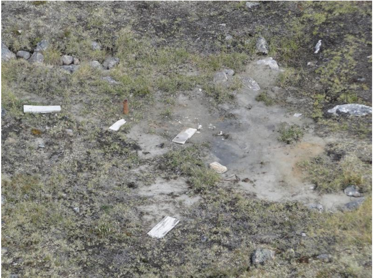
Figure 9. Drill hole with incomplete cleanup. N67°14'38.5" W92°59'04.8". Debris left on site and casings/collars not removed as per the licence. Also apparent that cuttings were not directed to a sump; rather they were left to accumulate beneath the drill.
