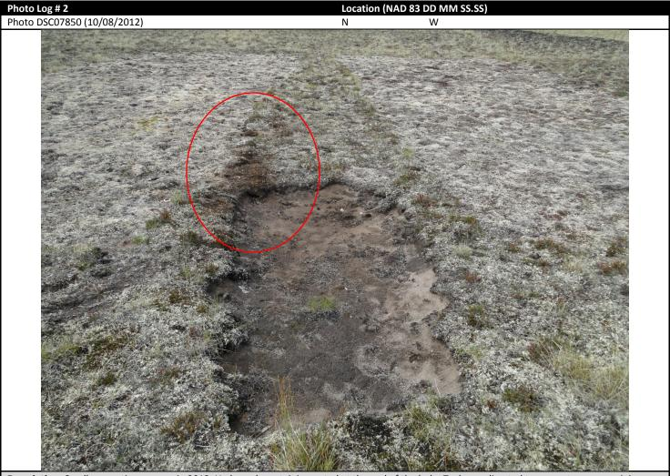
**Description:** Small excavation as seen in 2012. Hydrocarbon staining noted at the end of the hole; Teck was directed to excavate any remaining contaminated soil and backfill the hole.
