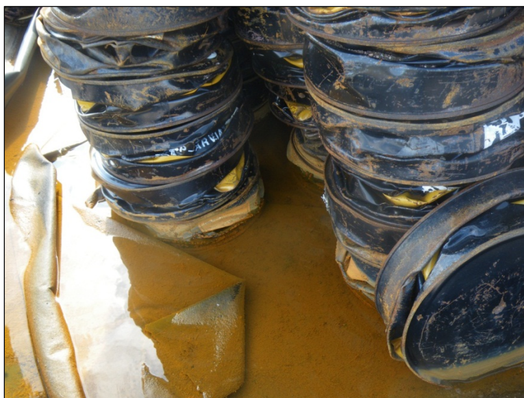
Plate 6. Standing water in crushed fuel barrels berm with amber colour and visible oil sheen.
