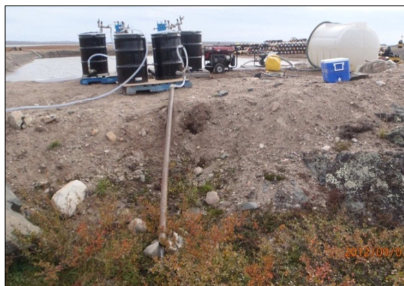
Plate 3. Oil water separator used to treat water pumped out of the fuel containment area. Water is pumped through pressurized vessels containing activated carbon.
