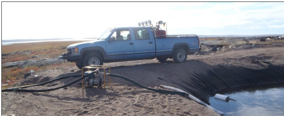
Plate 5. Hose and pump used to collect untreated water sample from the FCA being set up (not yet connected in this photo).
