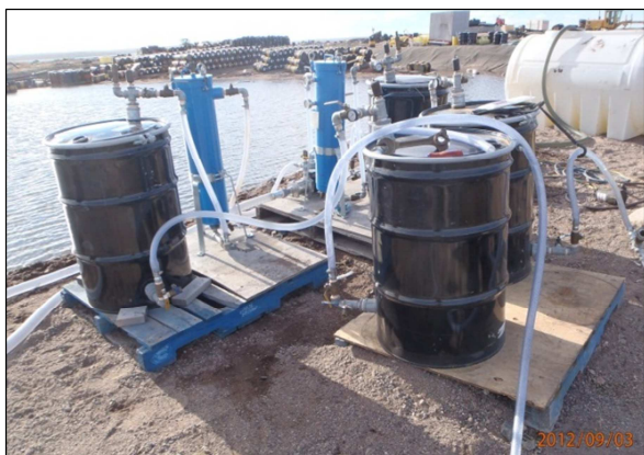
Plate 3. Oil water separator used to treat water pumped out of the fuel containment area. Water is pumped through pressurized vessels containing activated carbon.
