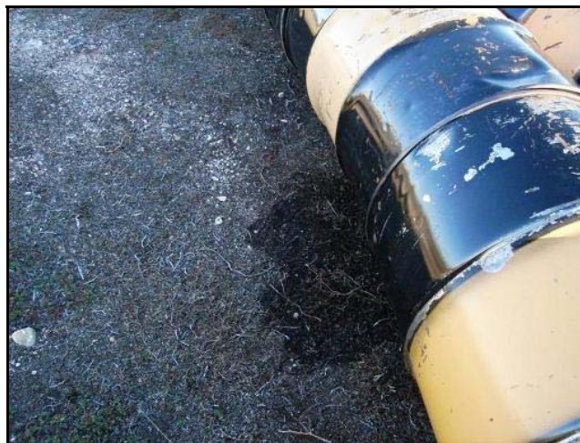
Plate 2.1-8. Fresh fuel leak from barrel (Airstrip 2).
