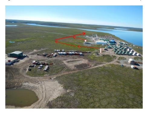
Currently, the greywater pipes discharge to a sump excavated in permeable soils within the active layer, underlain by permafrost. Discharged greywater both infiltrates into the active layer soils and overflows to wetland drainages that lead away from the camp (to the left in the photo) and eventually toward Goose Lake in the background in the approximate direction shown by the thicker red arrow. The minimum distance from the more northerly discharge to Goose Lake is in excess of 150 m.
