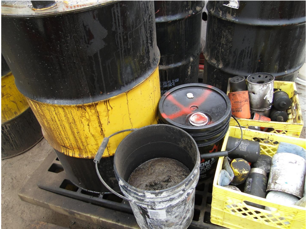
Figure 21. Open haz waste by Major shop. If pail overflows or falls, containment will not be adequate.
