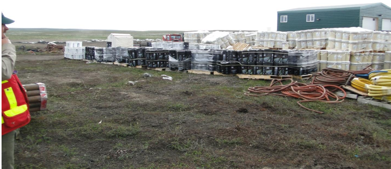
Figure 22. Stock of drill greases and additives to be stored in secondary containment.
