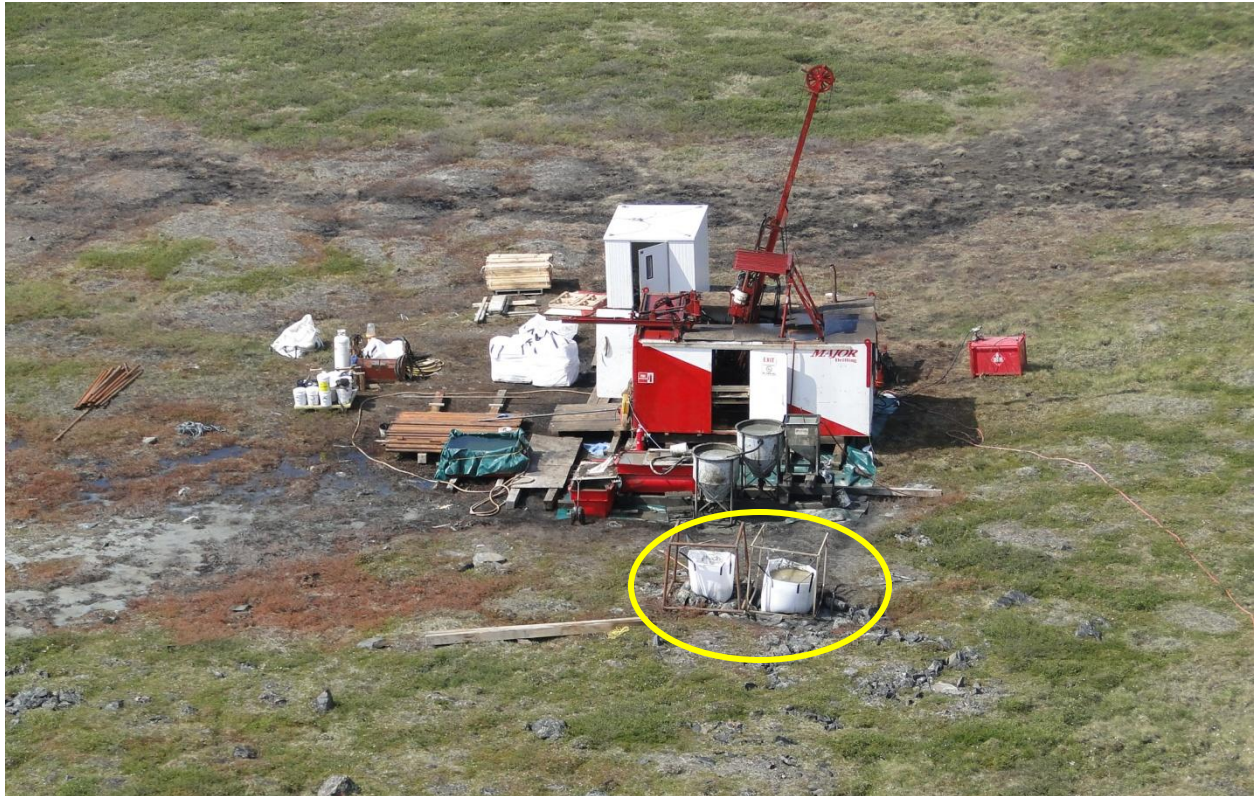
Figure 11. Current drill setup. Polydrill system and the use of mega-bags to capture cuttings are recent improvements. Mega-bags should sit in an appropriate rocky depression that will contain the water so it doesn't flow downhill.
