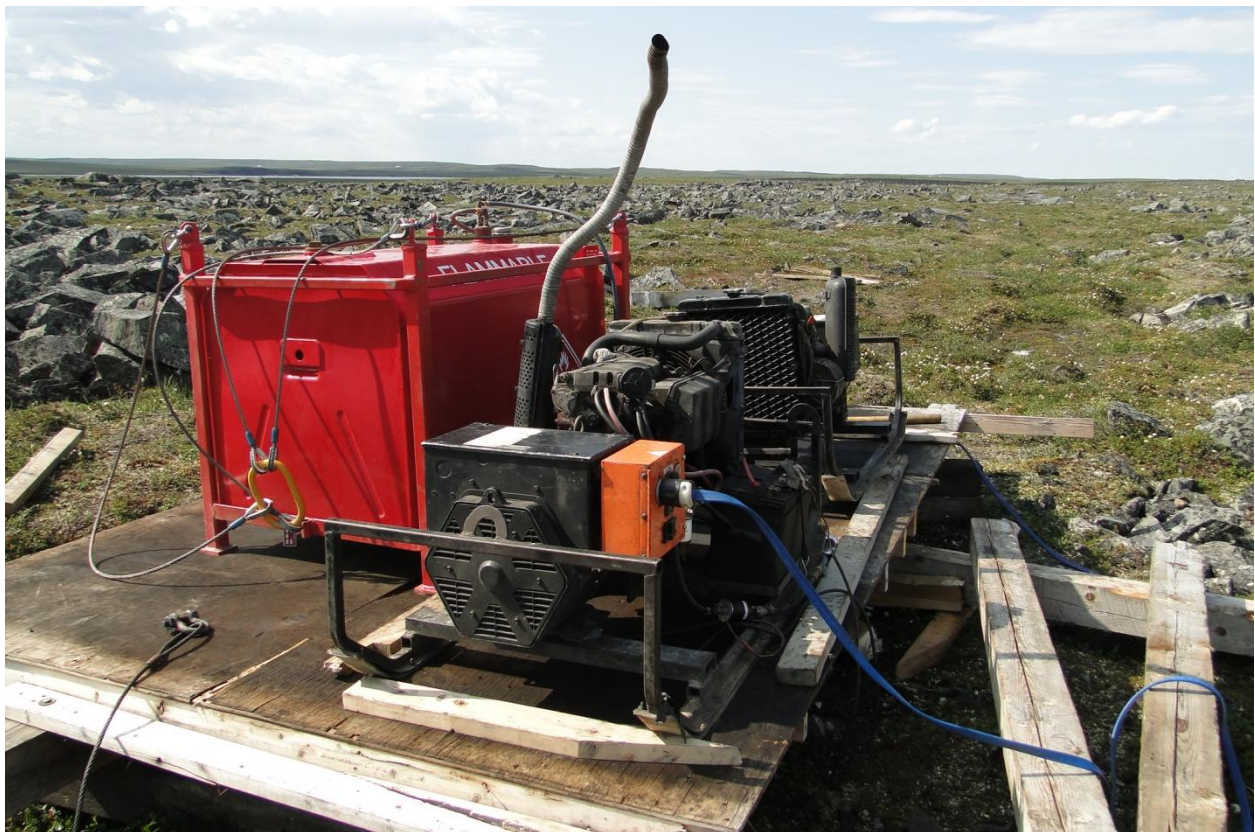
Figure 18. Fuel tank and pump should sit on a hard tray in case of spills or leaks.
