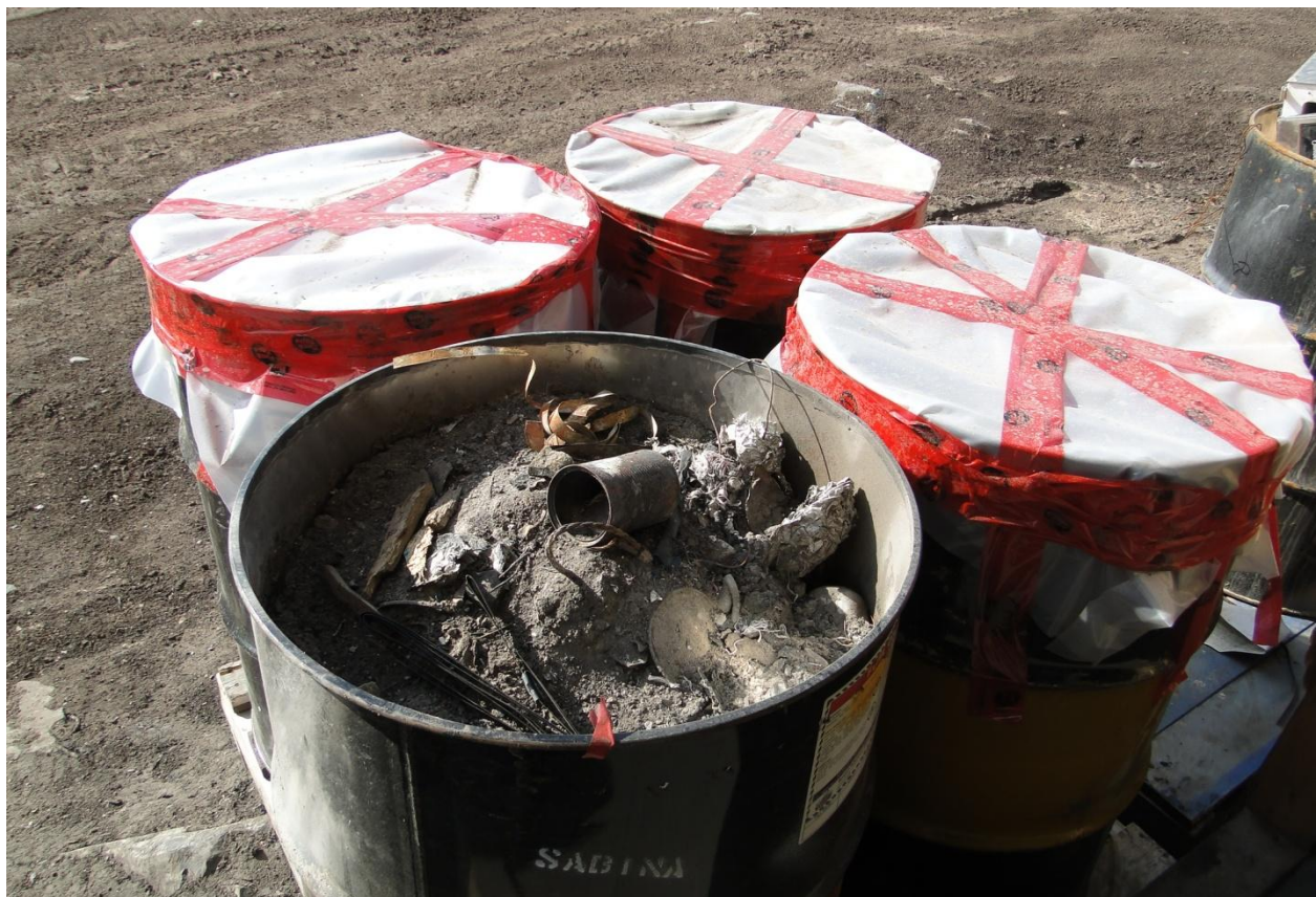
Figure 4. Metals and cable in incinerator ashes.
