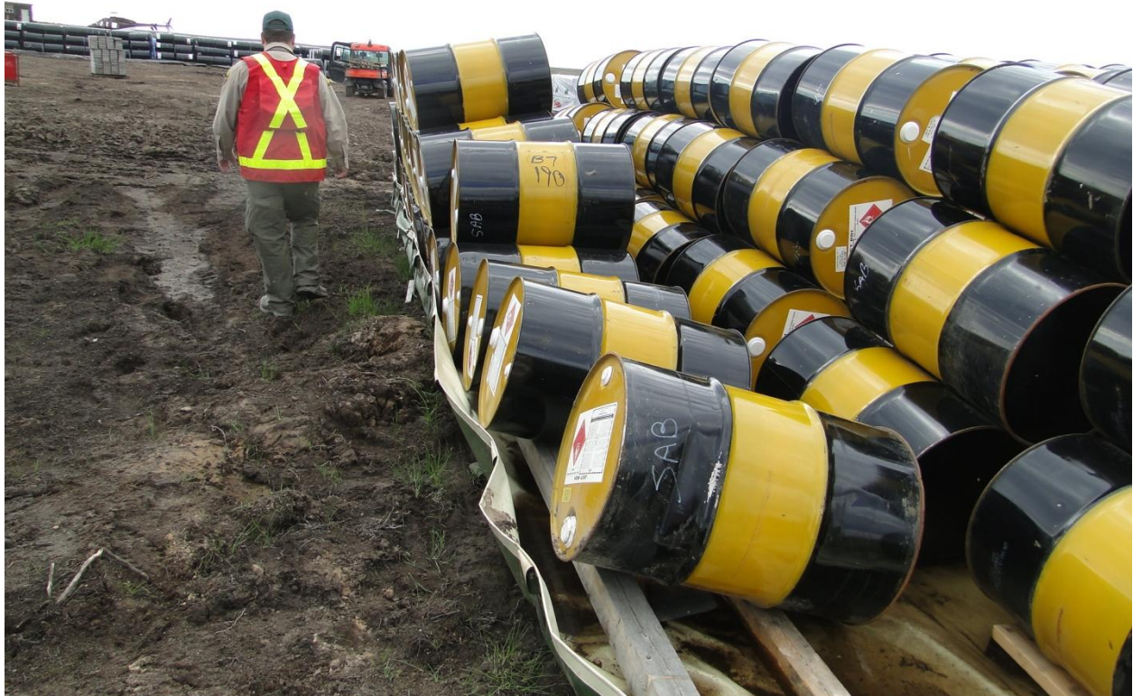
Figure 13. Piles of barrels stacked during winter shift and lean on soft ground. In this photo they lean right over the berm.
