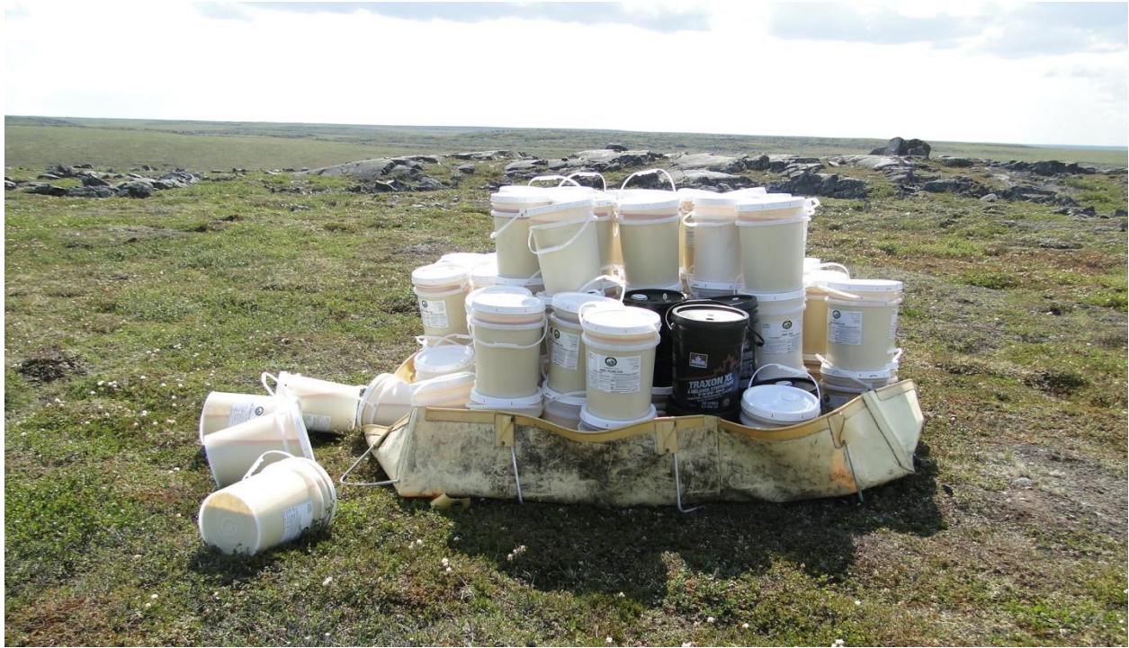
Figure 17. Pails of drill additives fallen out of collapsed containment.
