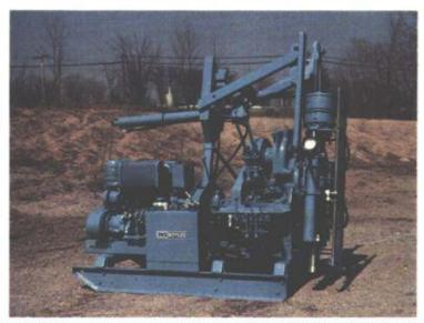
The BBS 25 is a medium capacity drill for holes of 590m (1950 ft) of B† wireline. The above drill is shown with an air cooled Deutz F4L912 diesel engine, H size swivelhead with swivel head guard, hydraulic chuck, hydraulic side-mounted wireline hoist, dual hydraulic pumps, and mast mounting base.
