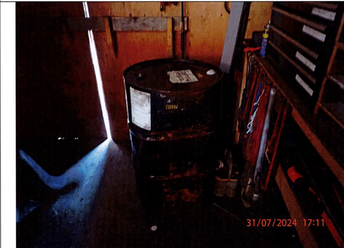
1 fuel drum outside of containment inside the mechanic shop
