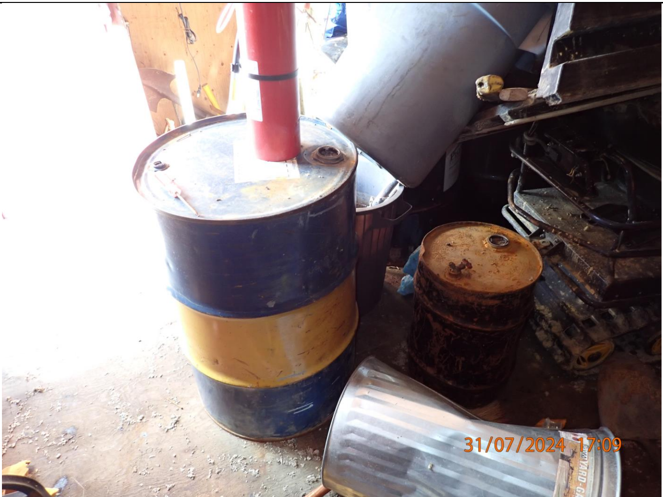
2 fuel containers out of secondary containment inside the mechanic shop.
