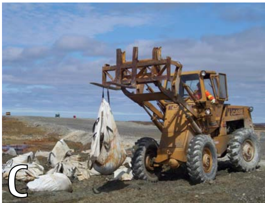
Photographs C & D: Picture C showing a mega bag lifted by the front loader, while picture D showing the bag sliced open to let the drilling cuttings out of the bag.
