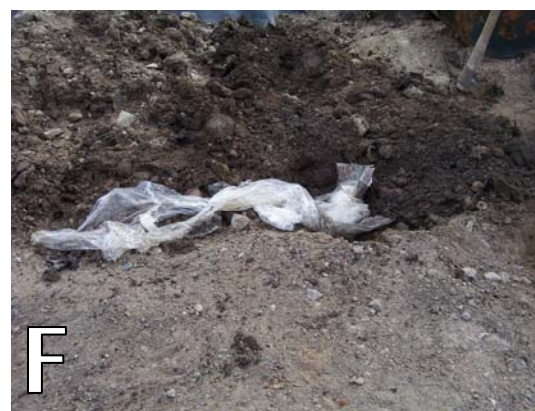
Photographs E & F showing non-biodegradable materials recovered during turning of the contaminated soil stored in the LTA at Boston Camp. Most of these products were plastics and absorbent pads.
