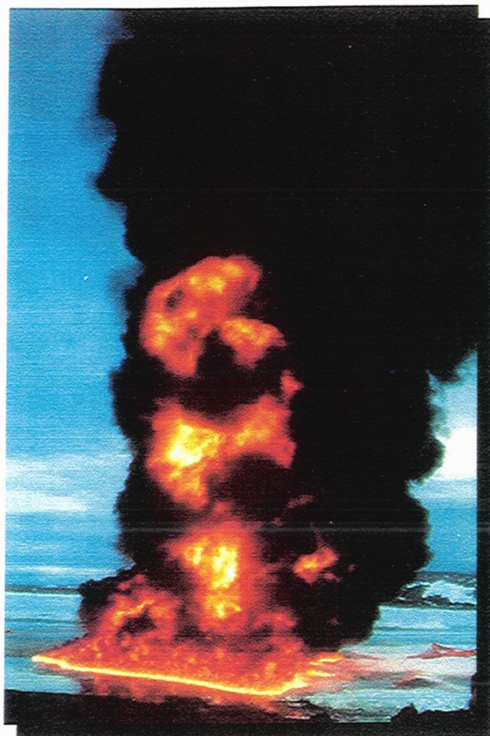
Photo 6 In situ incineration of liquid hydrocarbons on surface of water.
