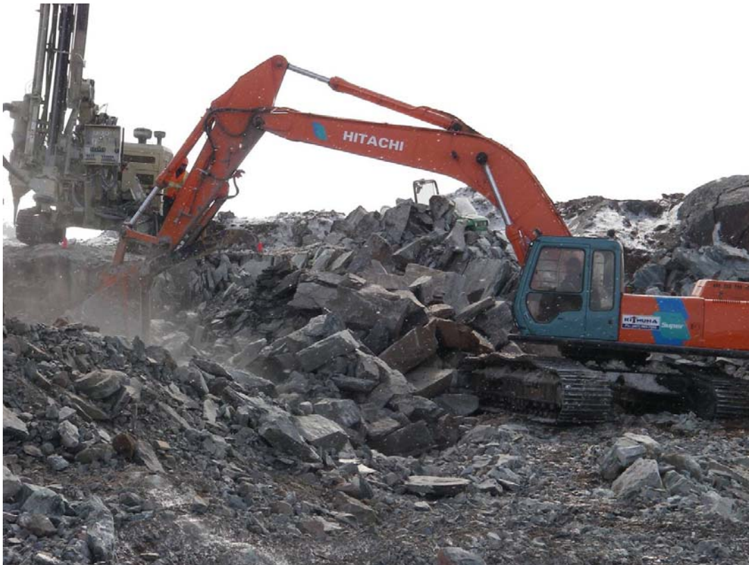
Photo 2: Large fragments produced from the blast due to wide spacing joint sets.
