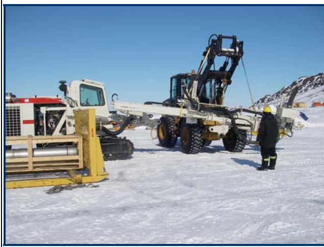
1. & 2. Terex mechanic attaching boom to R20C airtrack drill.
