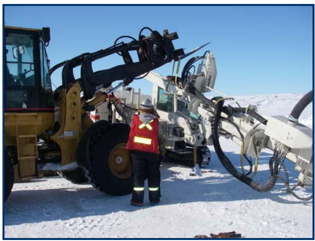
1. & 2. Terex mechanic attaching boom to R20C airtrack drill.
