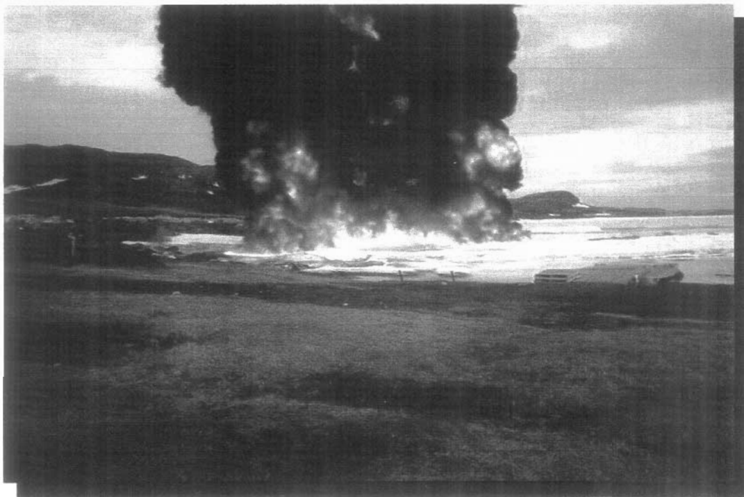
Photo 7 In situ incineration of liquid hydrocarbons on surface of water.
