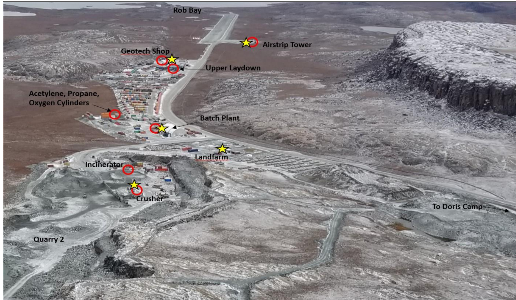
Plate A.3. Quarry 2, Laydowns, Airstrip (Note: Red circles are fuel or chemical storage locations, smaller containment locations may vary. Yellow stars indicate default spill kit locations.)
