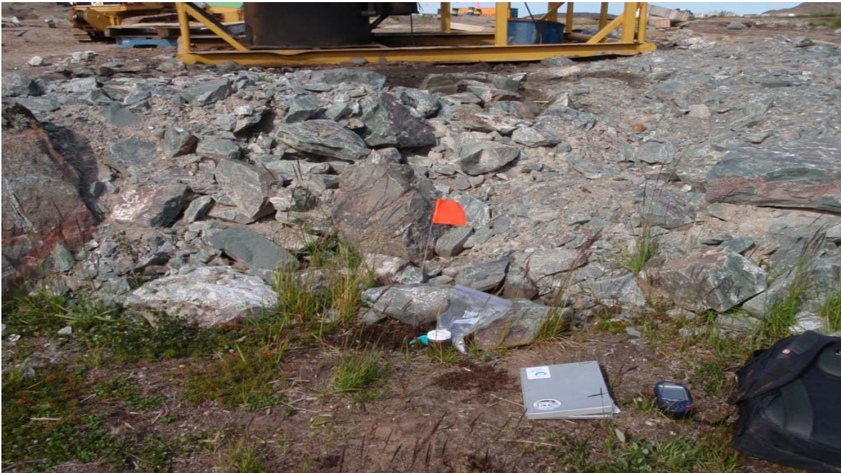
Photo 7: Sample PLF09-SS-084 collected south of the incinerator. There was hydrocarbon staining with sparse vegetation in the area.
