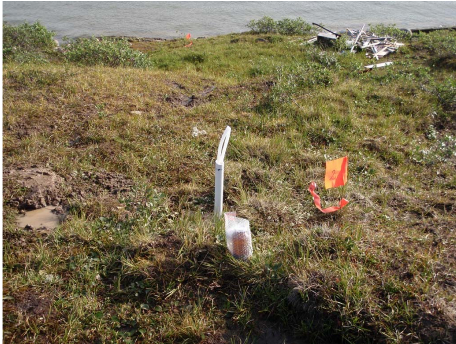
Photo 9: PMW -1 and Sample PLF 9-SS-038. PMW-2 installed in a drainage course downgradient of Areas 3 & 4.
