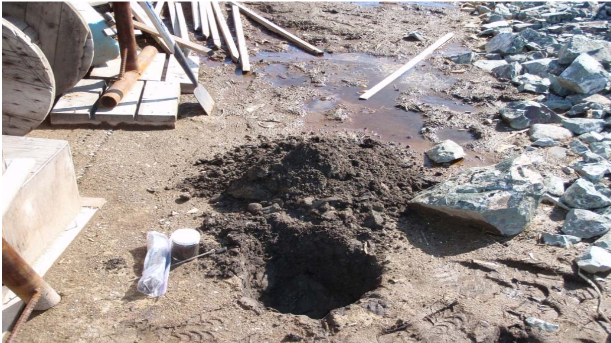
Photo 13: Sample WLF09-SS-026 at Area 1 Southwest of Former Tank Farm. There was hydrocarbon odour with anoxic conditions at the bottom of the test pit. Black stains visible around the area.
