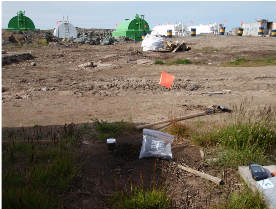
Photo 6: Sample PLF09-SS-082. Looking west with dark brown staining (1.5m X 1.5m) where the sample was collected in the foreground. Strong odour present.
