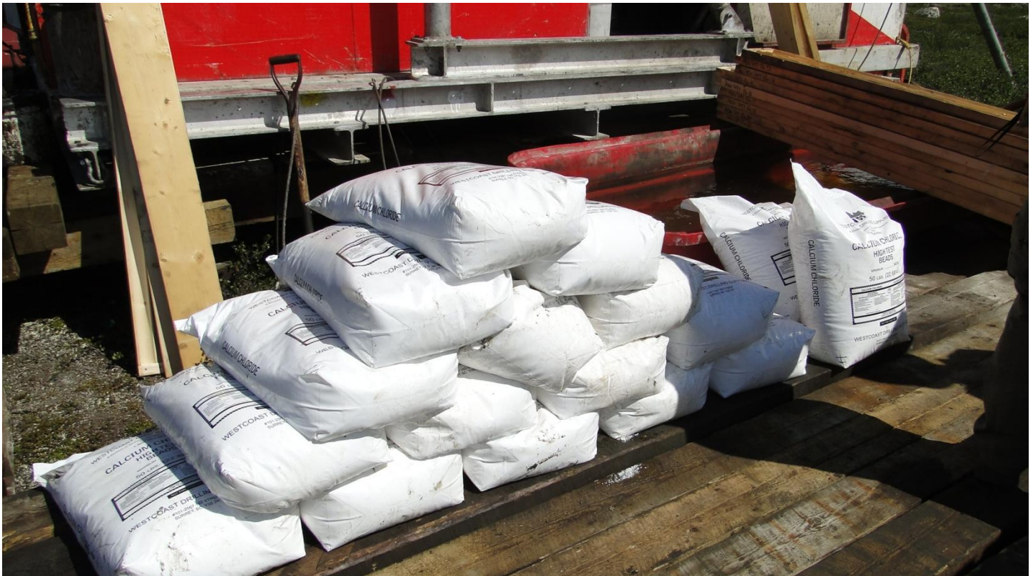
Figure 8. Salt stored without containment.
