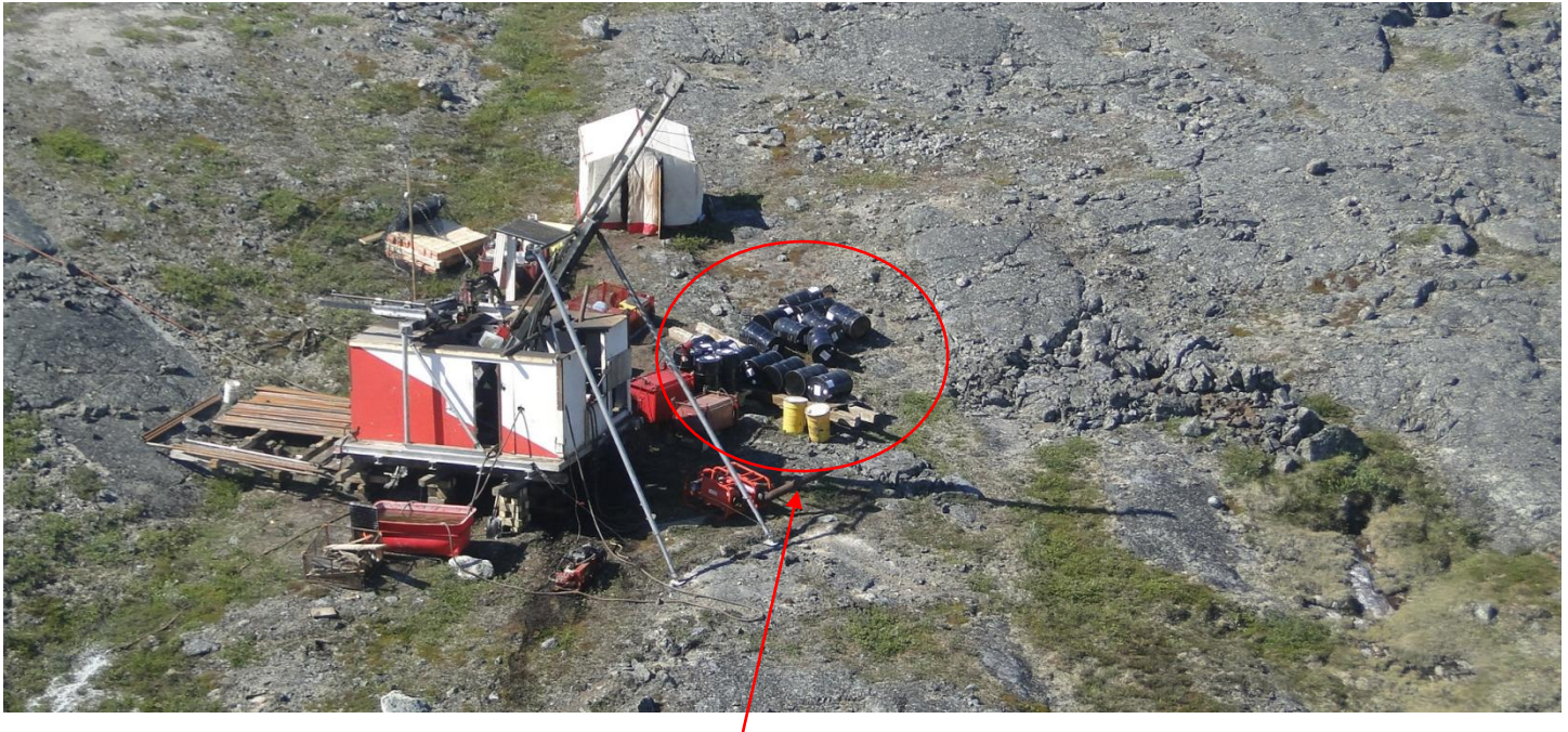
Figure 7. Drums held on timbers, sloped off the hill at a downward angle.
