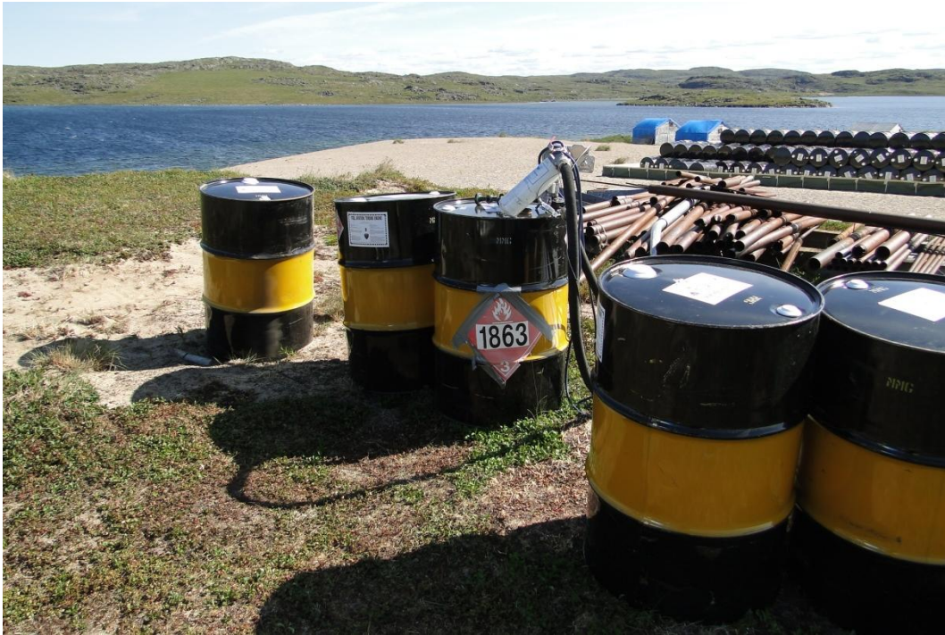
Figure 9. Hood helicopter refueling area - no secondary containment.
