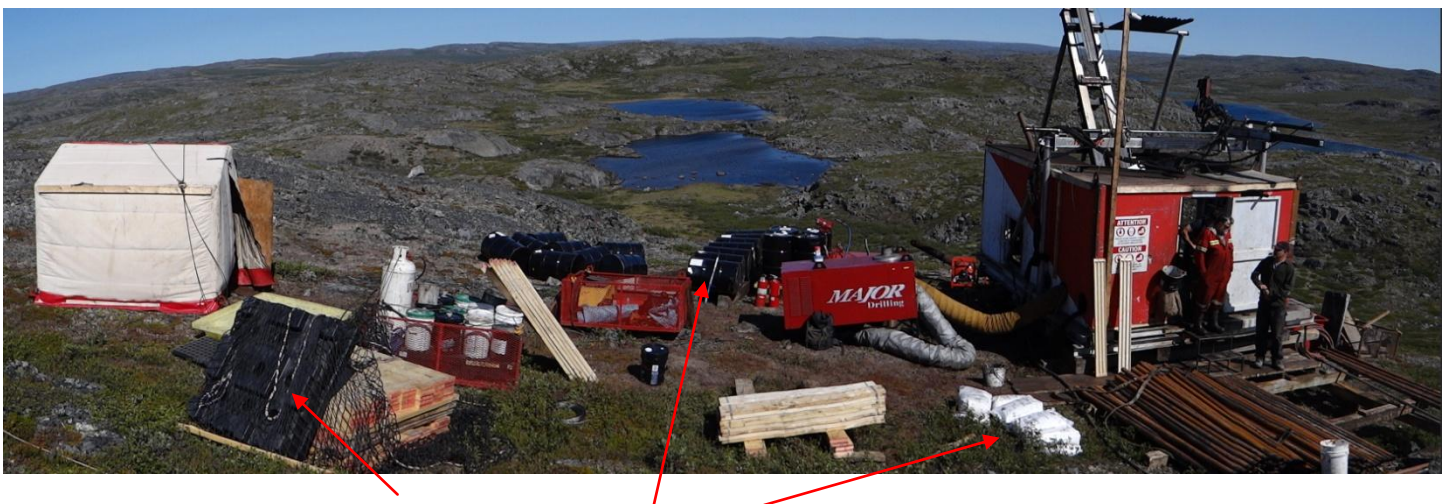
Figure 6. Drill 1493 setup - showing pallets sitting unused, while fuel and salts have no containment.
