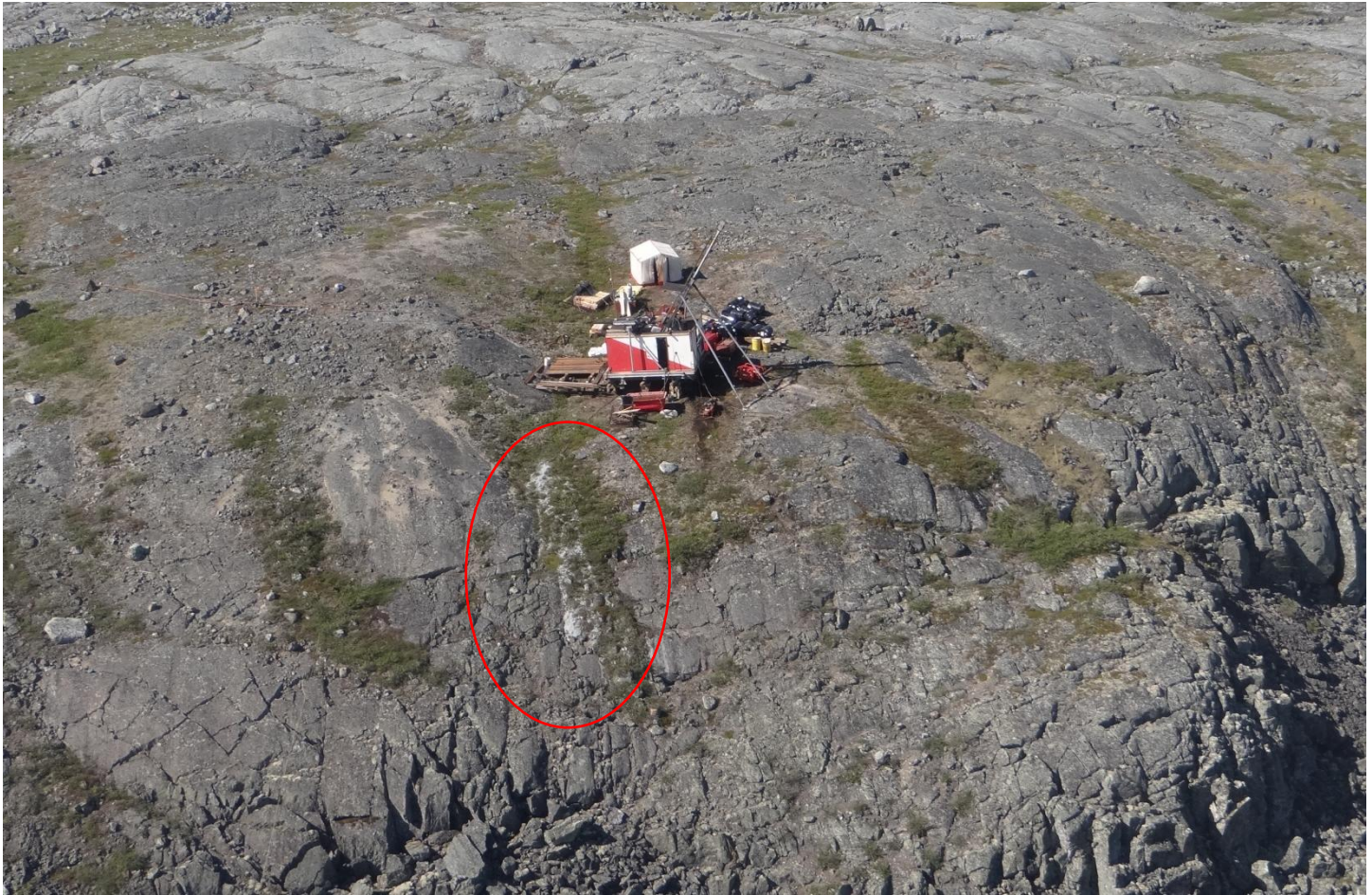
Figure 5. Drill 1493, with drill waste spilling down the side of the hill.
