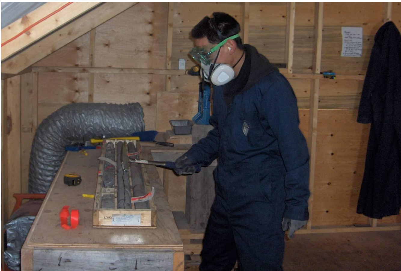
Photo 26 - Clifford Kreelak (Baker Lake Inuit hire) Splits Core
