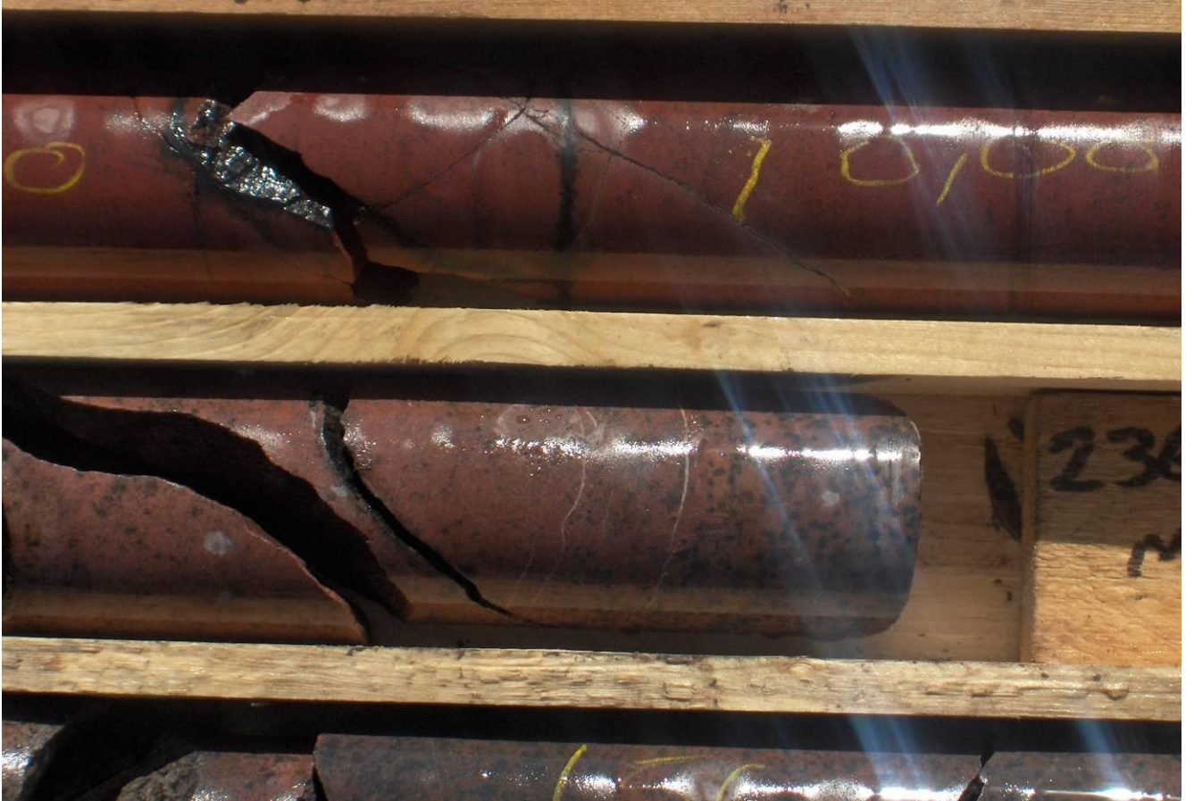
Photo 13 - Altered Kazan Sandstone with Pitchblende Fracture Fills (L7-07-08)
