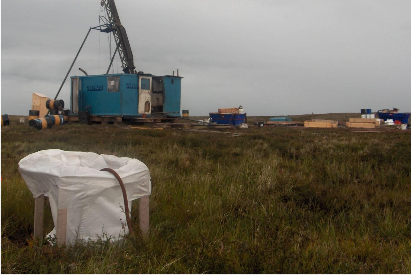
Photo 20 - KZ Drilling with Large Bag to Catch Rock Chips from Drill Return
