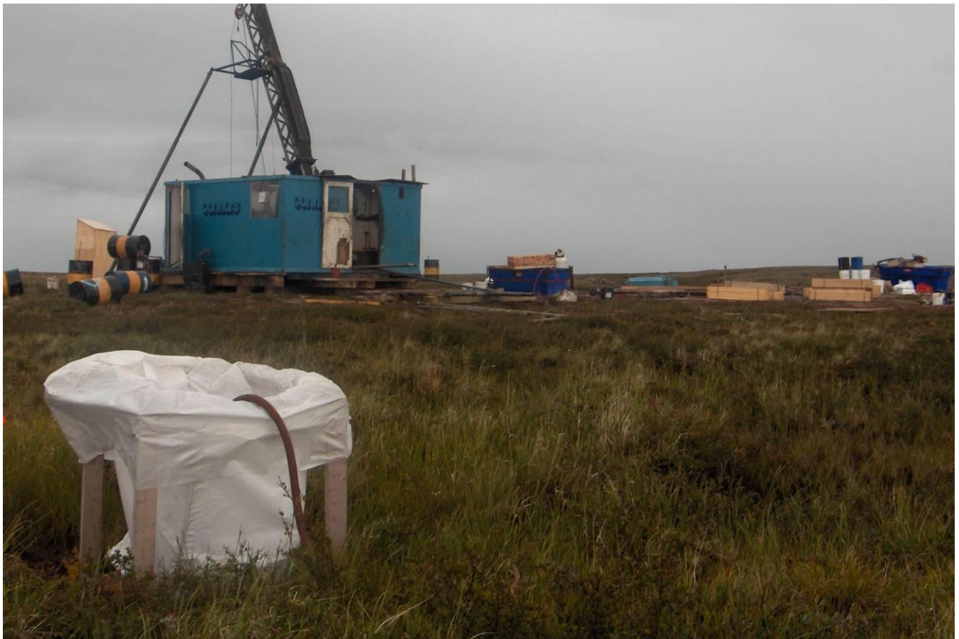
KZ Drilling : Large Bag Used to Catch Rock Chips from Drill Return
