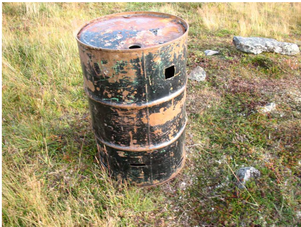
Photograph 5-2 Punctured Drum to aid Seepage
