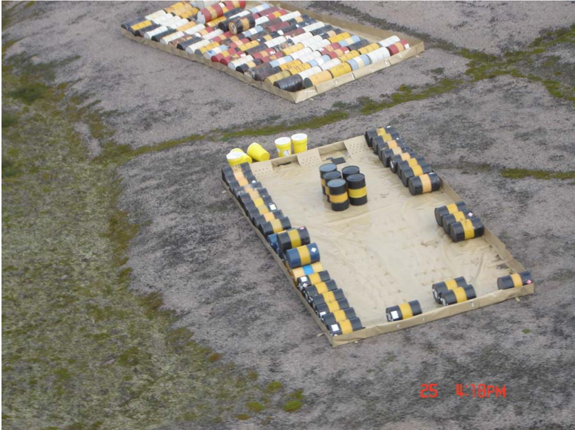
Figure 2.4: Fuel Cache at Esker with secondary containment
