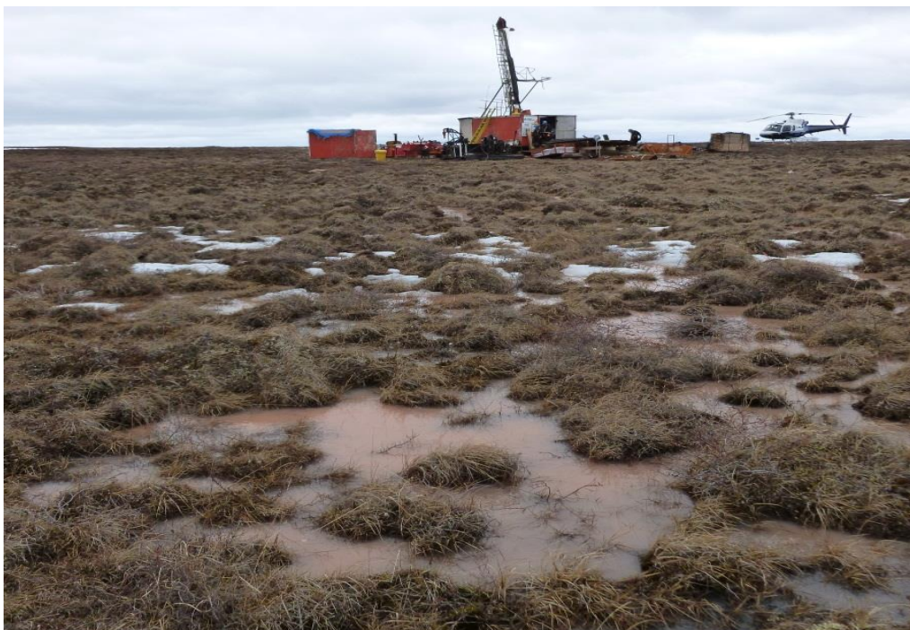
Photograph 3.4-5: Runoff Water Mixed with Drill Cuttings June 17, 2015
