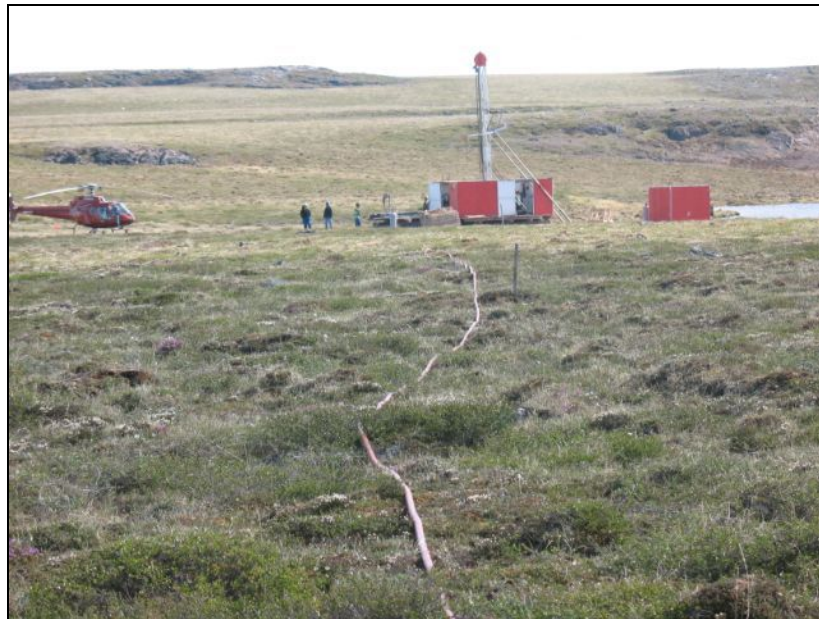
Figure 7 – Set-Up END-08-03 showing the discharge hose that runs 600 feet away from the drill
