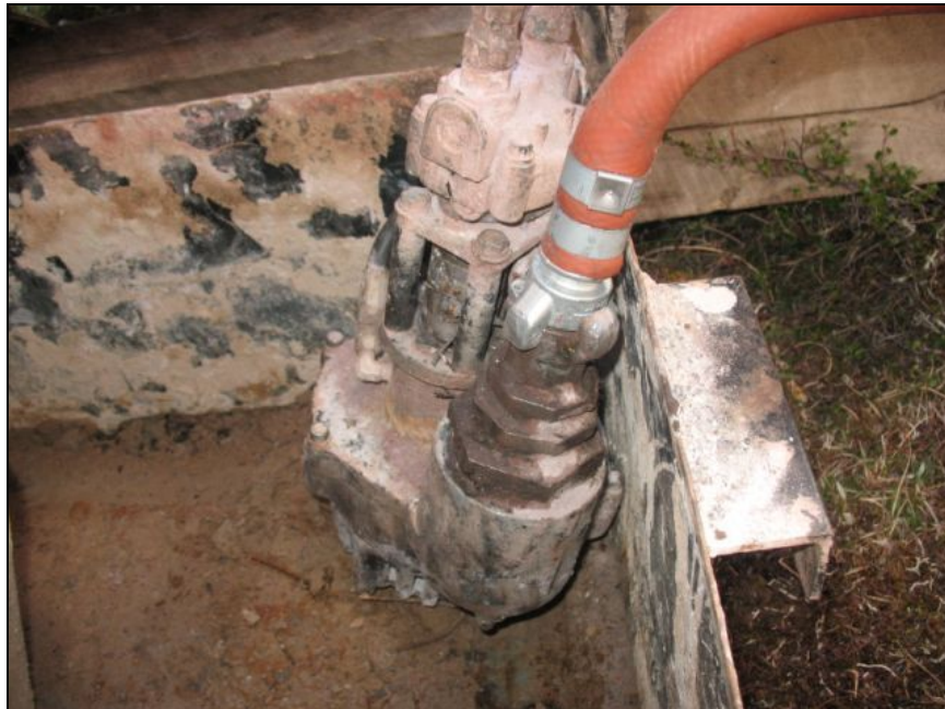
Figure 6 – Set-Up END-08-03 showing the containment and sludge pump
