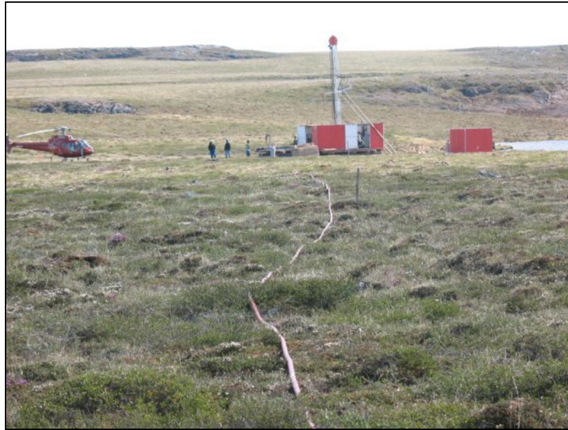
Figure 11 – Set-Up at END-08-03 showing the non-radioactive cuttings discharge hose
