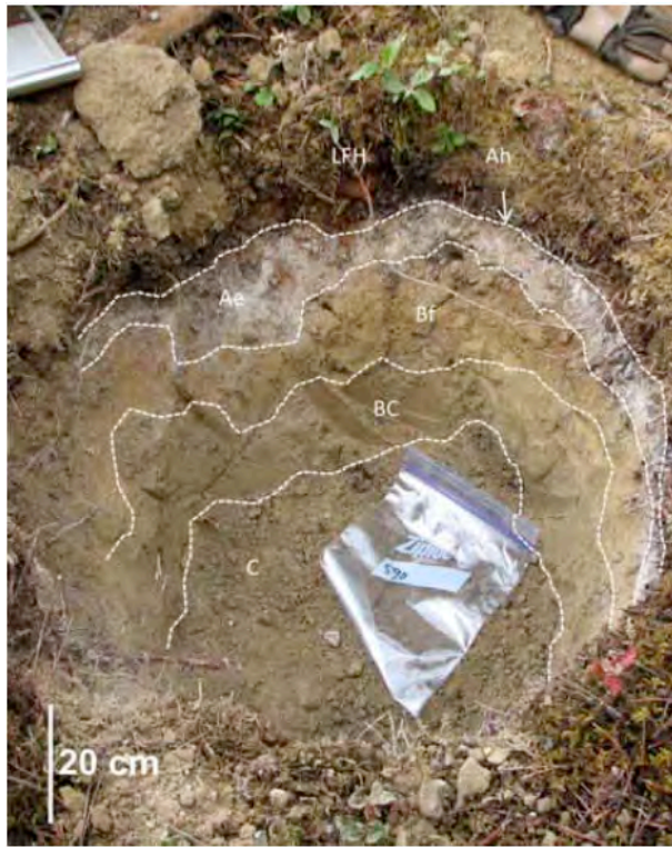
Figure 5— An example of a hole dug for soil or till sampling. Hole is approximately 50cm across and 40cm deep. Holes are backfilled after the sample has been collected.
