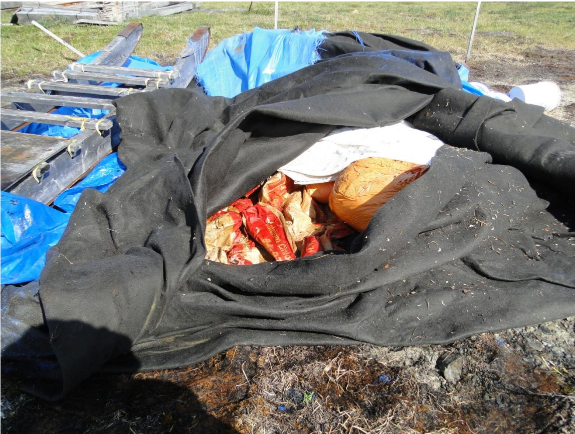
Figure 4. Contents of tarped pile – CaCl bags: wet and contents dissolved.
