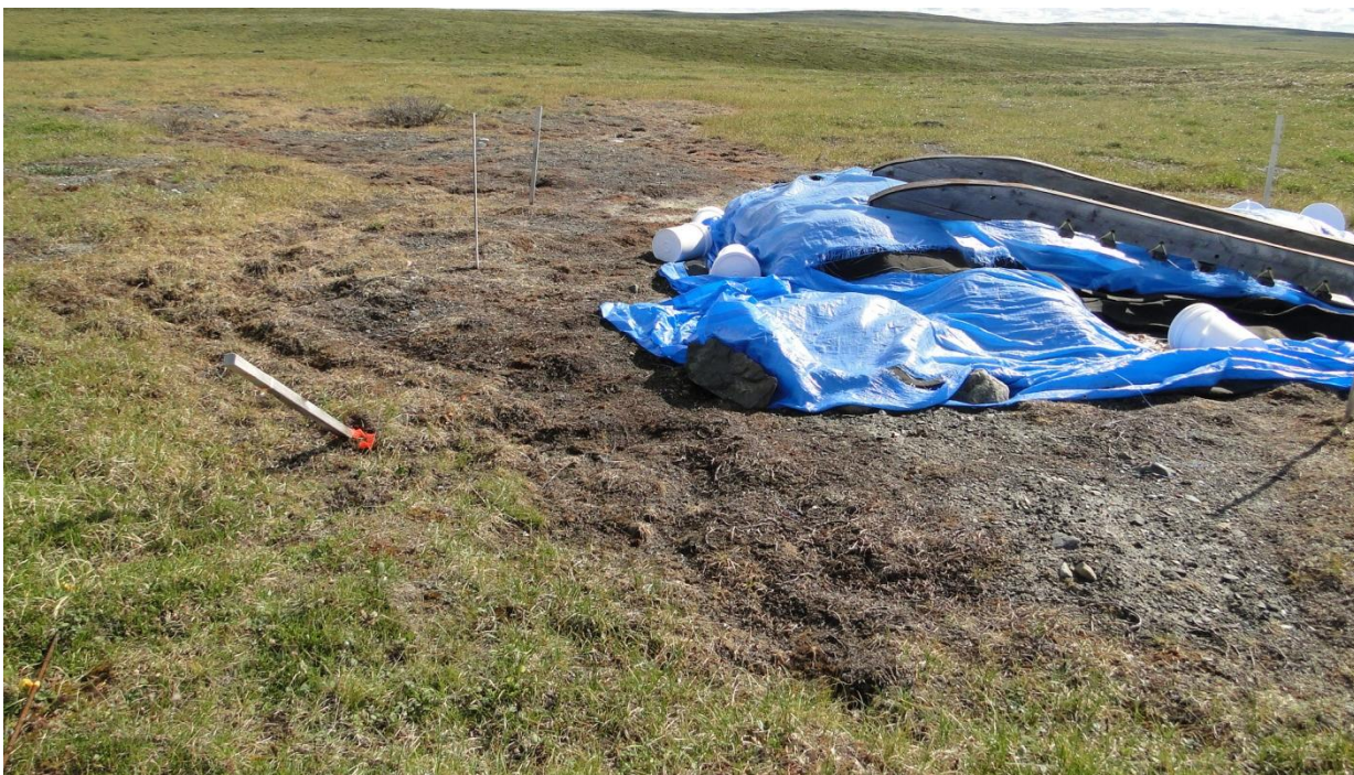
Figure 3. Dead vegetation and reddish colour characteristic of a salt burn.
