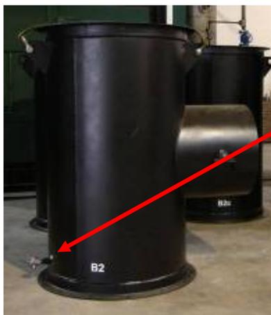
3. Stack Thermocouple on Stack
