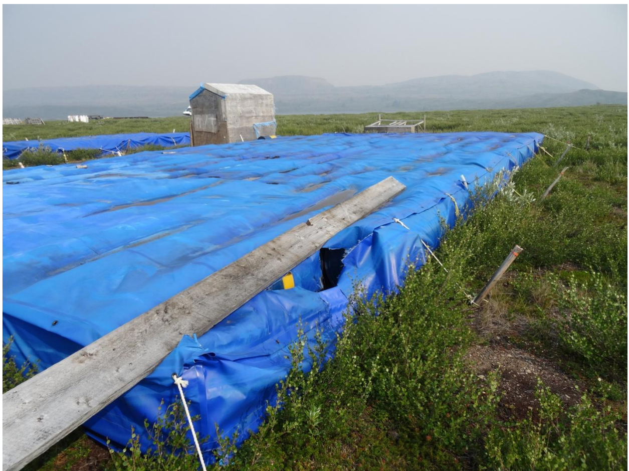
Figure 10. Berm covers are damaged. Cap was left off and (potentially contaminated) water drained out.
