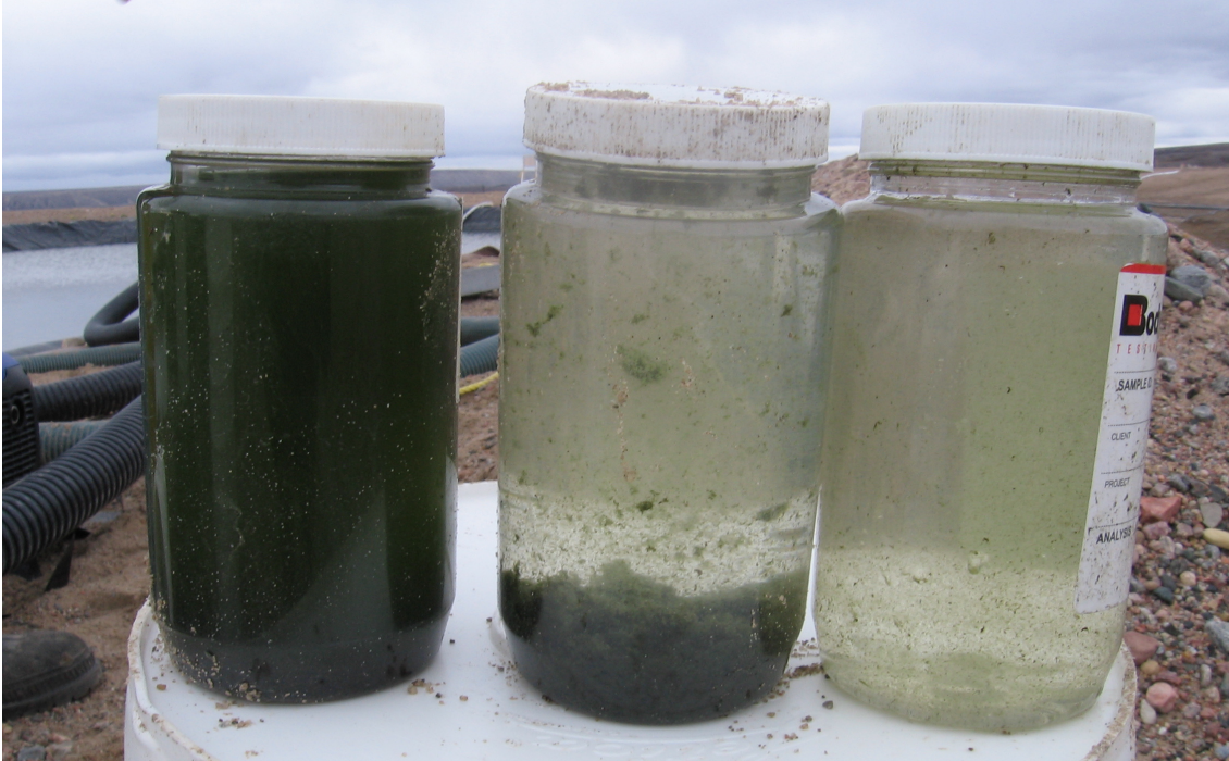
Photograph 3 Geotube test results (L to R: Raw PWSP No. 1 sludge, coagulated/flocculated sludge sample, Geotube filtrate)
