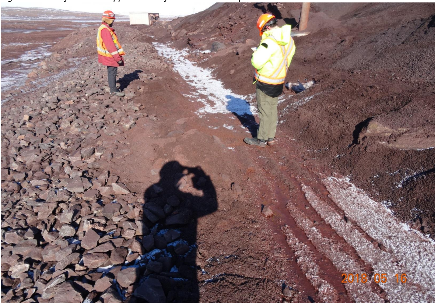
Figure 2: Debris from what appears to be from the Ore Stockpile in the ditch near the “E-house”
