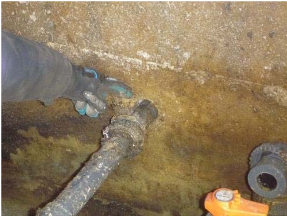
Photo 2 – Initial cause of spill- separation of O-ring from fitting
