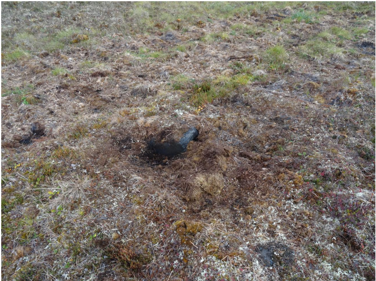
Figure 10. Closer view of hydrocarbon stain at b). Strong hydrocarbon smell remains in the humic (organic) layer.
