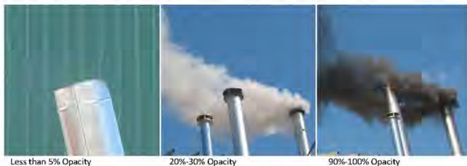
Figure 6 - Examples of Smoke Opacity Ratings
