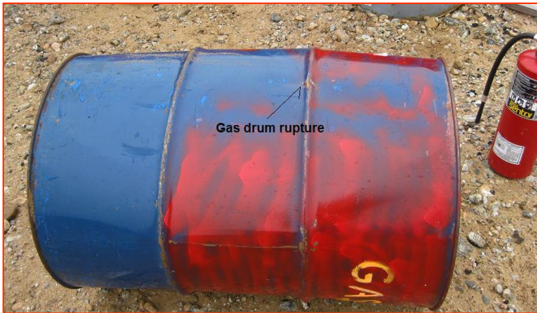
PHOTO 5: REFILLED PETROL DRUM WITH RUPTURE, NANUQ CAMP, NU
