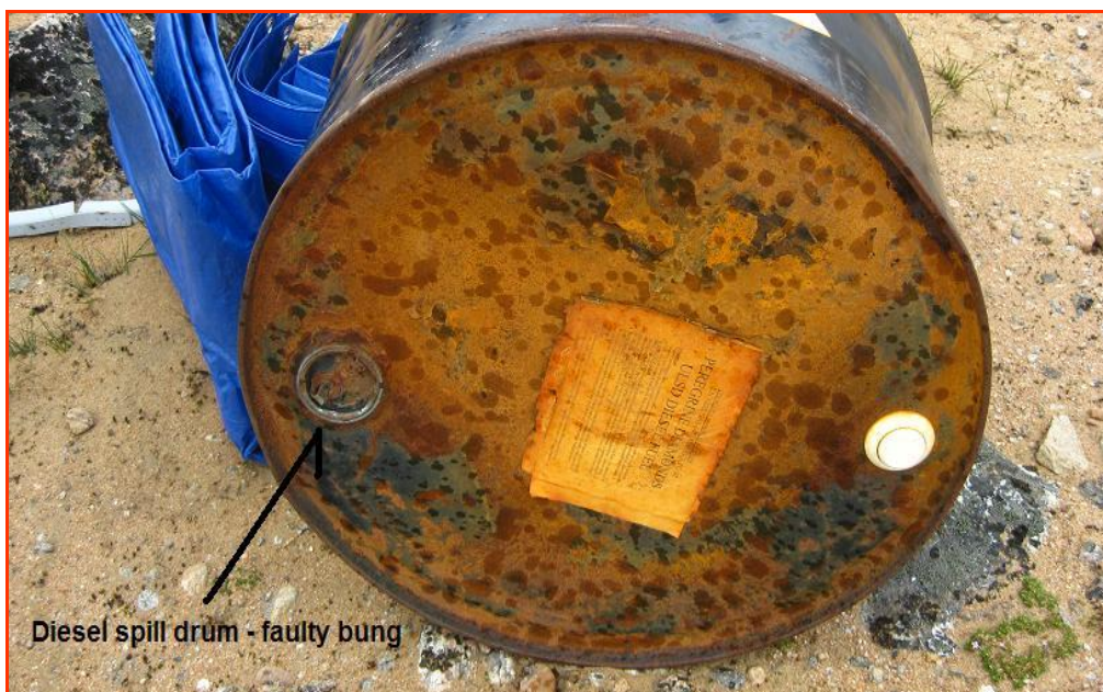
PHOTO 3: CLOSEUP OF FAULTY BUNG ON REFILLED DIESEL DRUM, NANUQ CAMP, NU
