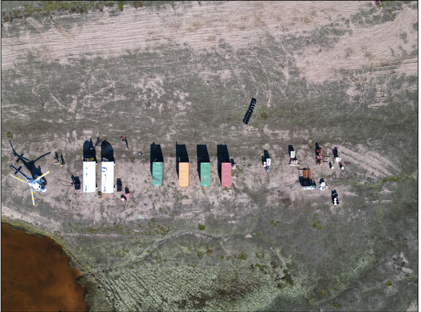
Figure 2-3 Layout of the staging area at the Loki airstrip. Two 50,000 L fuel tanks holding Jet A and diesel are located on the left side (south) and there are four seacans storing drilling supplies.
