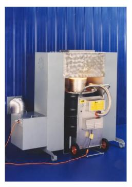
The SmartHeat works in conjunction with the SmartAsh by capturing the heat being emitted by the incinerator and directing it into buildings using a blower unit.
