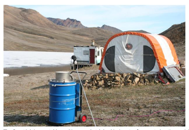
The SmartAsh is a portable, multipurpose batch load incinerator for remote locations, mining camps, job sites, oil drilling operations, truck stops, construction sites, islands, barges, campsites and military installations. Waste materials are loaded into a drum, once ignited the lid is placed on the drum and a whirlwind of fire is created by the high velocity blowers creating a clean combustion.
