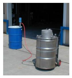
Oil Away is an option that allows the Smart Ash to burn waste oil. It is delivered with an electrically operated dosing pump, delivery hose and spray rail that fits inside the drum.
