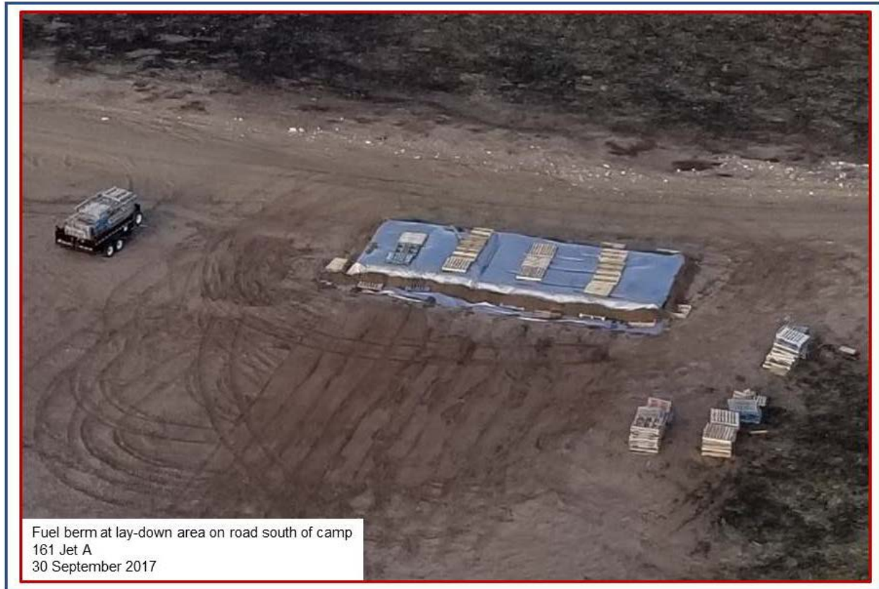
Figure 5. Aerial view of the fuel berm, at a road accessible staging area, with Jet A-1 fuel stored for the winter
